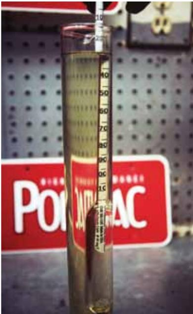
**5** Though Rockett Brand Racing Fuel supplied specific gravity for each fuel, we confirmed the specification using a hydrometer.
