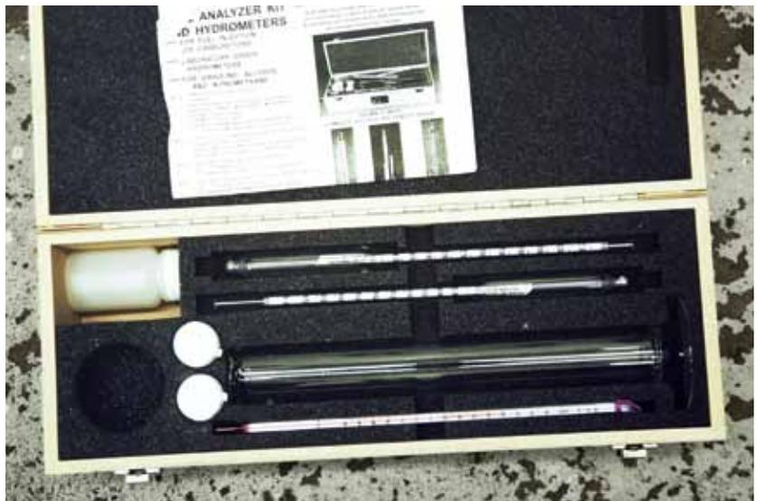
**3** Kinsler offers a very complete fuel test kit to measure the weight of the fuel. It is a good tool for the serious racer.
