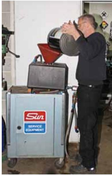
**6** Bob Wise loads the dyno fuel cell with fresh Rockett Brand Racing Fuel. It's a process that would be repeated often throughout the day. Each time the fuel was changed, the system was purged to ensure that there was no residual fuel from the previous test remaining.
