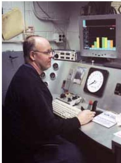
**7** Craig manned the dyno controls for each pull. With the Depac data system and controls the testing was uniform to guarantee accurate results.
